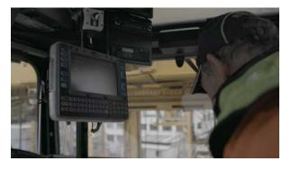
In an environment that is rough and demanding, warehouses, manufacturing, and intermodal industries may find that they are constantly replacing damaged mobile computers that are not suited for shock, vibration, and just overall rough environments. Most mobile computers are also not suited for deep freeze conditions, such as a cold storage with temperatures dropping to -30C.
