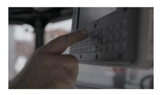
Data collection and entry are a breeze with the physical, full 64-key QWERTY keyboard, number pad, and 10-function keys. The key functions are also programmable to address specific use cases. The keyboard supports ANSI 3270 & 5250, and the touchscreen has resistive and capacitive (PCAP) options. The touchscreen and keyboard are easily replaceable for on-the-go maintenance.
